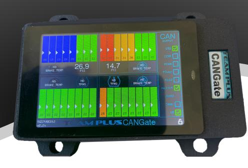
Display and connect Team Plus sensors to your existing CANbus dash logger using the Team Plus CANGate. CANGate connects to the Team Plus Wheel Turtle, Team Plus TPMS and Team Plus Brake Turtle (\*) sensors over Bluetooth and then passes data onto your CANbus, so it is available to any CAN based dash or logger or ECU.
